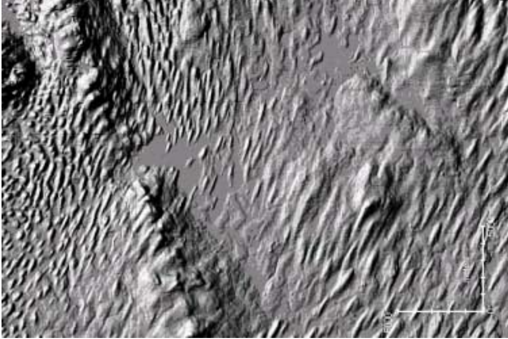
Figure 5.2a and b Hillshaded DEM of Lough Gara, Ireland, using an illumination azimuth parallel (left) and orthogonal (right) to the principal lineament orientation. Note the dramatic changes in lineament morphology, particularly above the centre of the image. Arrows indicate the azimuth angle.
